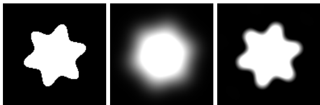
Figure 7: Left plot: Original image defined via flower-shaped characteristic function. Center plot: Blurred flower image obtained by convolution with kernel h(x, y) = e^{-100(x^2+y^2)} . Right plot: Deblurred flower image obtained by solving (49) to time T = 0.3 with \epsilon = 0.1 , c = 0.01 , \Delta t = 0.0002 , and \alpha = 10^4 .
